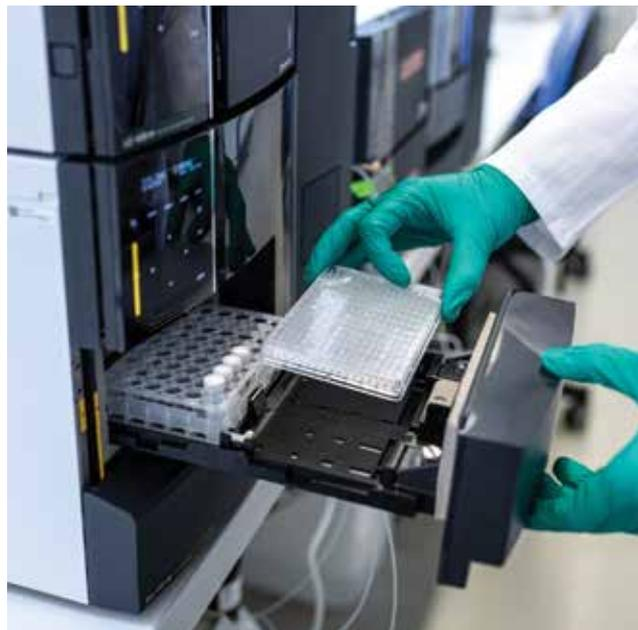
▲ **Figure 3.** An engineer from c-Lecta prepares an enzyme reaction in a 384-well microtiter plate for high-performance liquid chromatography (HPLC) analysis, which has become a standard tool for industrial enzyme development.
